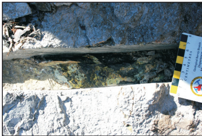
Plate 1. Uranophane-stained fractures within lapilli tuff developed proximal to the sample site, which assayed up to 13.8% \text{U}_3\text{O}_8 ; Powe prospect.
