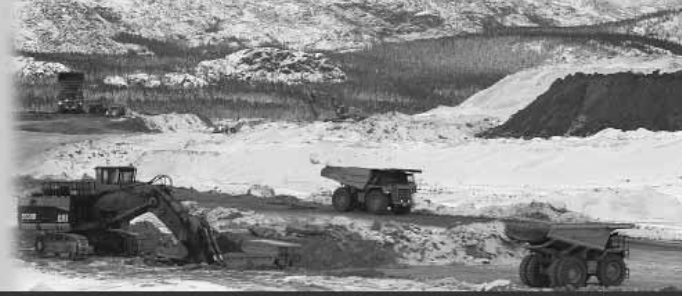
Prestripping of overburden on top of the ovoid deposit
