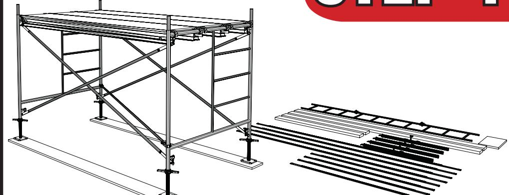
Install the second cross-brace to both the frames. Next you need to level and plumb the scaffold. Start at the high point of the scaffold. If possible, use the jack-nut to bring the highest corner down closer to the sill. Next bring all four corners up to that point. If the bottom cross-members of each frame are level with each other, the frames should also be plumb.
