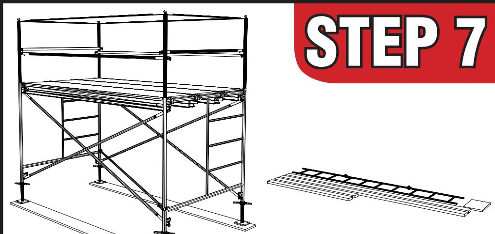
Attach the guardrails to the posts on all the exposed sides.
