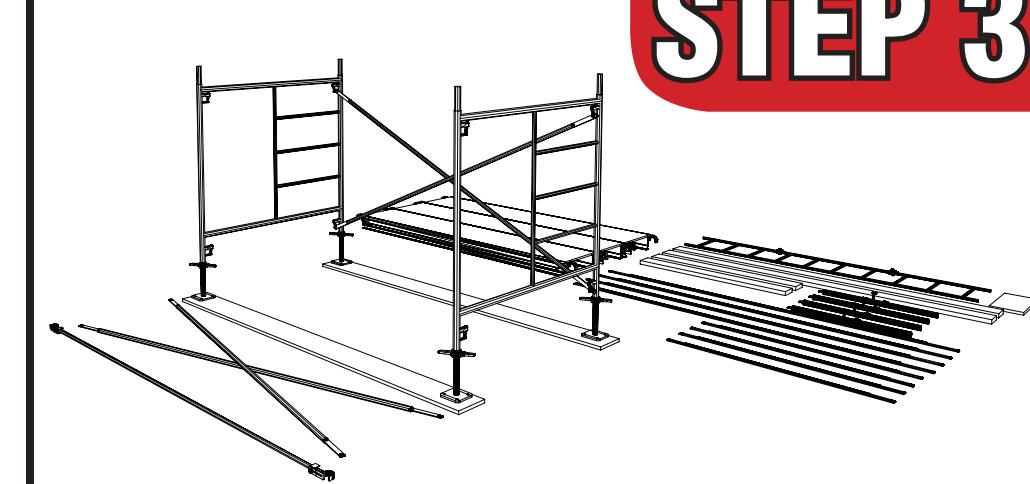
Install the second frame onto the base plates. Secure the first cross-brace to the second frame.
