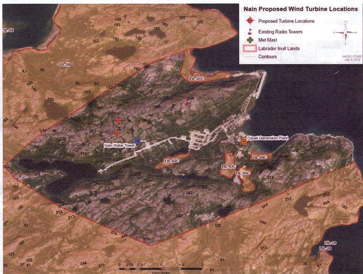
The proposed location of the project's wind turbines on Nain Hill, above the water tower, is right on the edge of an area zoned as Residential for future residential development. The illustration below shows the proposed location of the two wind turbines, T1 and T2 (ignore the white line around them—they just show the general area affected by the turbines). The access lane to be built from the water tower to the turbines' location is shown as a red line approximating the lane's alignment.
